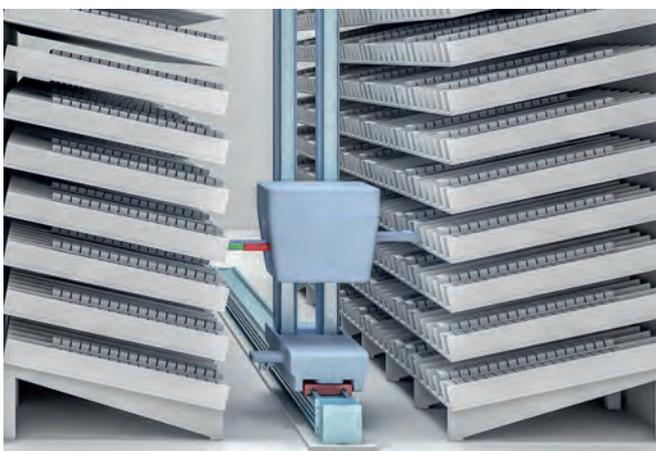
Fig. 3 - In automated warehouses, telescopic rails extract parts from the shelf and load them onto the carriage, or vice versa.
