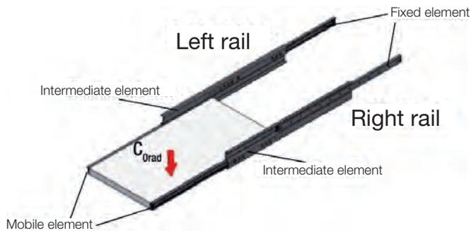
Fig. 2 - Diagram for correctly mounting of a pair of telescopic rails. The horizontal configuration is often recommended.
