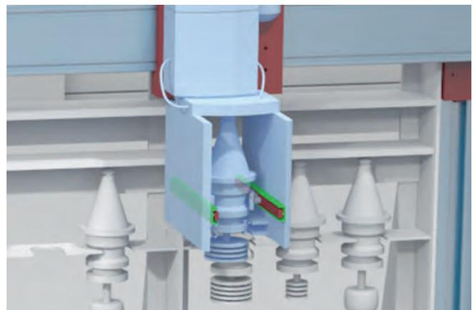
Fig. 1 - Tool changer: a bilateral stroke enables the telescopic rail to extract the tool and position it in CNC machine.
