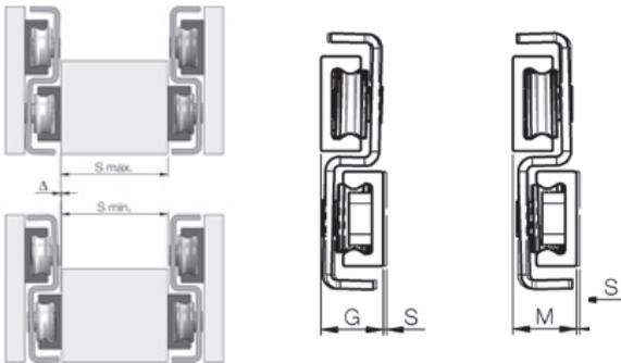
Fig. 5 - Telerace telescopic guides from Rollon can manage misalignment of the assembly surfaces thanks to axial floating rollers.
